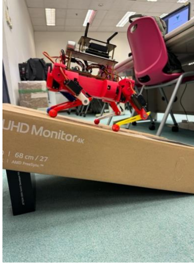
Figure 3.14: robot balancing on sloped surface with unlevelled body
