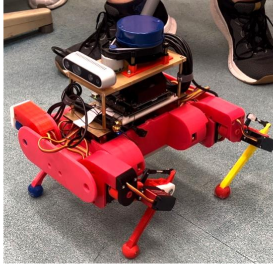
Figure 3.2: robot installed with a planar LiDAR and power bank
