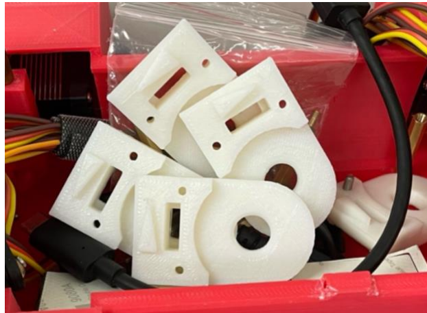
Figure 3.5: printing results of upper shoulder joints
