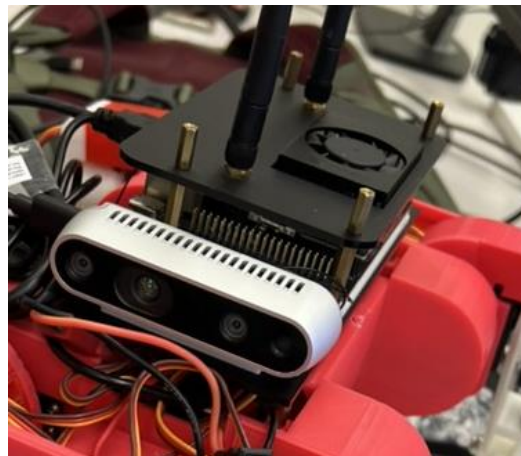
Figure 3.9: Final model design with laser-cut acrylic boards and copper stands
