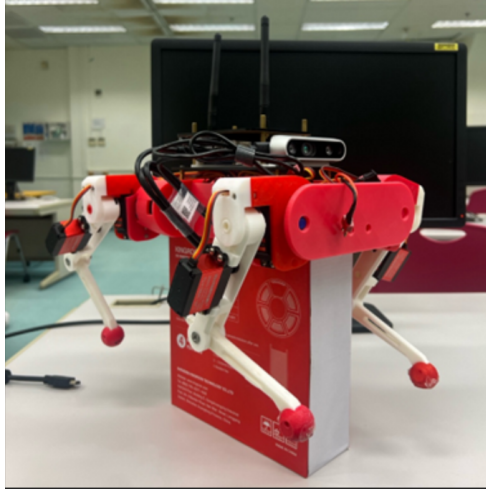
Figure 4.2: Quadrupedal robot with Jetson Nano, stereo camera, and lithium battery
