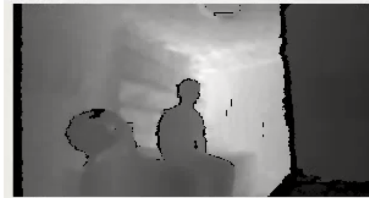
Figure 3.9: Depth image obtained from Intel Realsense depth camera
