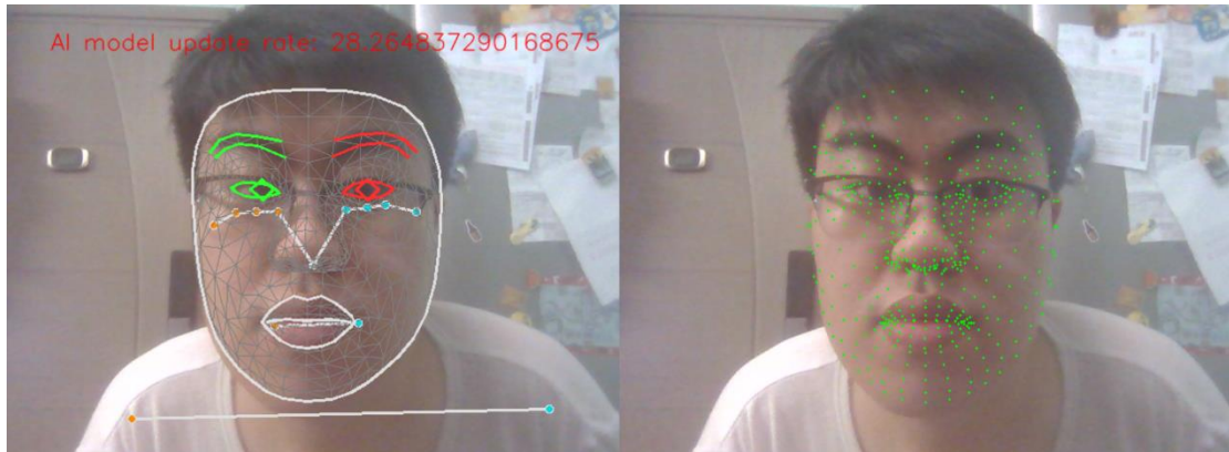
Figure 15: Example of filtering applied on landmark data (Filtered data on the right).
